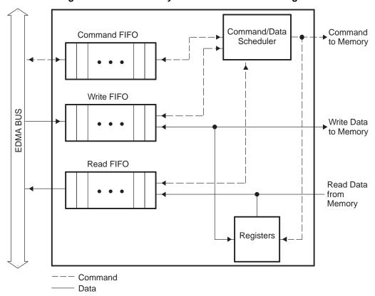
Figure 15. DDR2 Memory Controller FIFO Block Diagram
